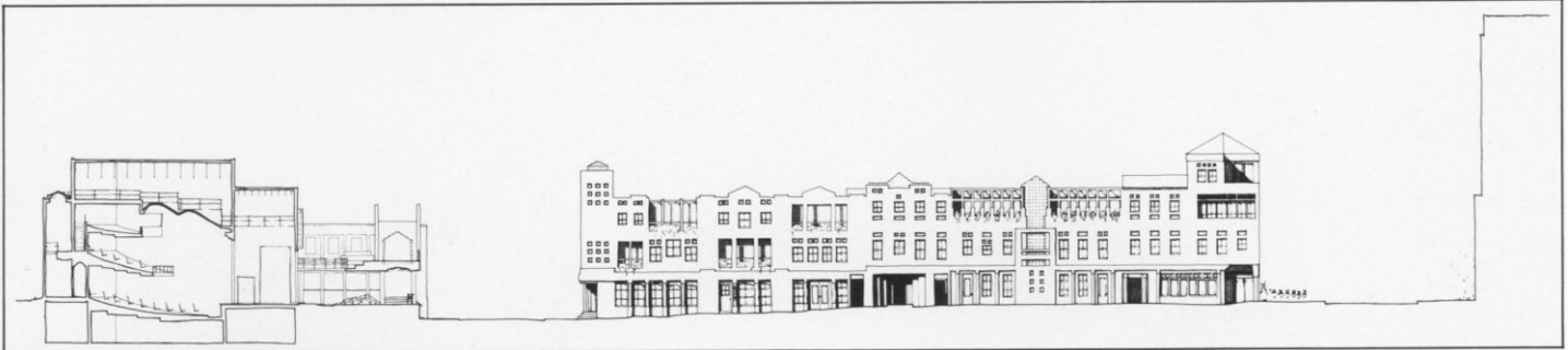
3 SECTION (Fall 1983). This section cuts through the main pedestrian street with the new community theatre on the left and the existing Center for Performing Arts on the right. Students: Matt Beahm, Peter Califiura, Susan Strange.
